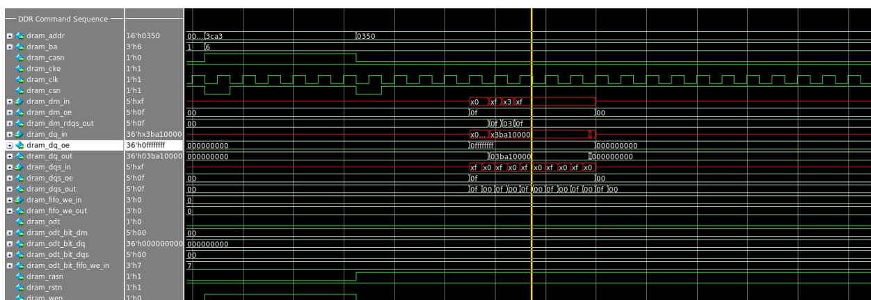
Figure 1-18. DDR Controller Command Sequence for a Single AXI Write Transaction
